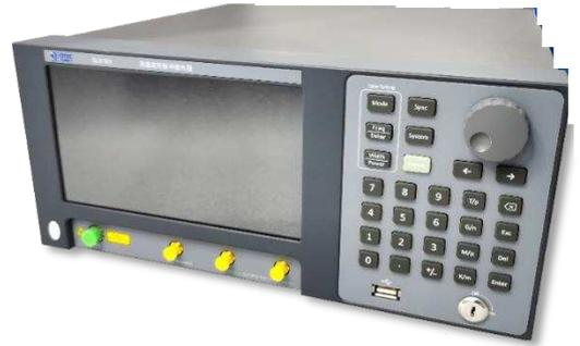
With built-in EVOA and PD, the optical power can be adjusted easily and shown on the screen for quantum optical applications. Besides pulsed laser mode, continuous wave mode is also supported, of which average power can be set and monitored as well.
